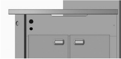
Typical 2nd thermostat and switch installation
