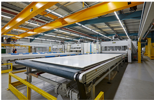
'SMART' GRP sidewall during the production process.
