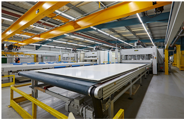
'SMART' GRP sidewall during the production process.
