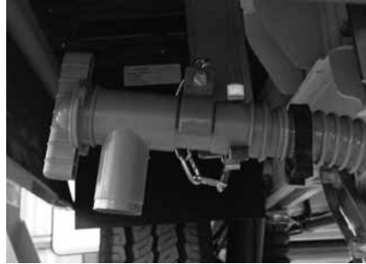
External view of suspended valve
