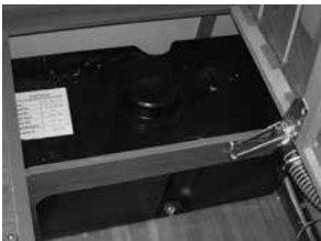
Escape fresh water tank showing central cleaning hatch
