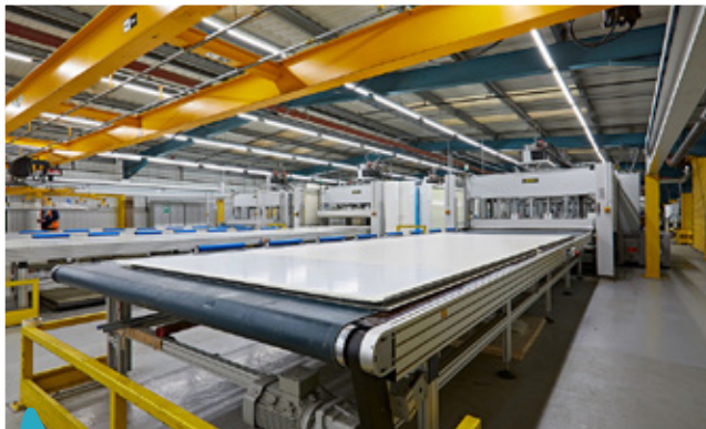
'SMART' GRP sidewall during the production process.
