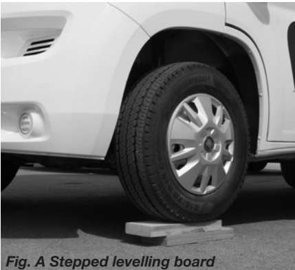
Fig. A Stepped levelling board
