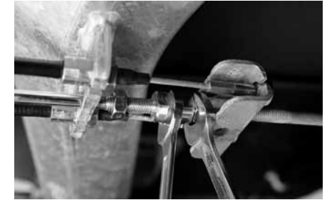
Unscrew push rod from brake rod and slide it from the guide tube. Remove the locking nut from push rod using two 17mm spanners.
