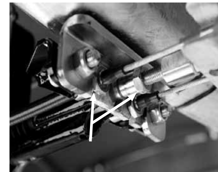
Using a 17mm spanner, slacken locking nut on push rod away from Bowden cable abutment as directed above.
