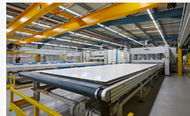
'SMART' GRP sidewall during the production process.
